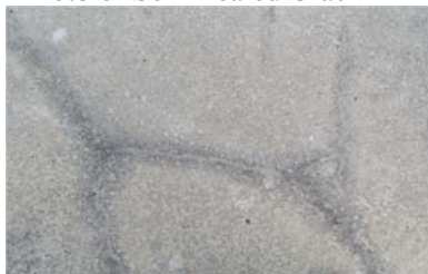
Photo of Self-Healed Crack
